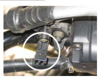
For the 2010 model year, a new type of clutch switch is fitted that has a two way latched plug. The switch is located directly under the clutch lever near the pivot point. This connector (arrowed in the photo below left) comes from the rear into the clutch switch. Cruise control MCS 6690/2 will fit these bikes.
