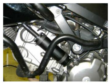
The Cable Interface Unit (3) is mounted on the fairing frame on the left side, beside the forks. The mounting bracket is clamped to the frame using hose clamps. The photo below shows the CIU with the fairing off the bike. The photo at right shows the CIU viewed from above inside the fairing. It has a new cable (4) running from it to the throttle bodies.
