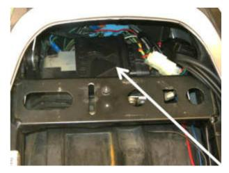
The Electric Throttle Servo (2) is mounted on the left side of the bike, under the seat fairing panel. The photos below show the bike with the seat fairing fitted (left) and the servo mounted to the frame without the panel fitted (below right). A cable connects it to the CIU (3).
