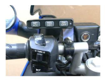
If risers are fitted to the handlebars and the switch contacts the fairing screen during steering movement, an alternate switch mount is available to allow the switch to be installed under the handlebar (5b).
