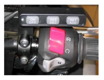
NOTE: - The size and mounting arrangement of the left side switch gear and handbrake on the DCT bike make it impossible to safely mount the control switch on left handlebar.
