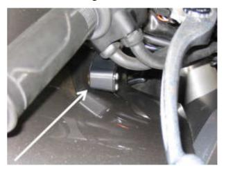
If you wish to mount the Control Switch (4) above the handlebar on the DCT version, a replacement control switch bracket can be supplied in the kit at no extra cost. This bracket may also be purchased as a separate item if desired. The part number of this alternate bracket is MCS830B.
