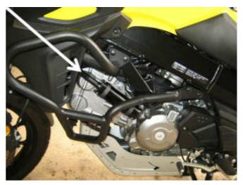
The CIU or Cable Interface Unit (3) is mounted on the fairing frame on the right side, beside the forks. The mounting bracket is bolted to the fairing frame using an existing bolt hole. The photo below left shows the location of the CIU behind the right side fairing panel, the photo below right shows the CIU with the fairing off the bike. The photo further below right shows the CIU viewed from above inside the fairing. It has a new cable (4) running from it to the throttle bodies.
