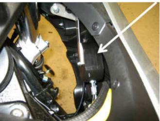
The Control Switch (5a) is mounted on the left hand (clutch) lever mirror mount. The switch is located above the left switch block. This photo shows the standard bracket, which allows plenty of room above the menu buttons for a gloved finger or thumb. We recommend this bracket unless you have particularly small hands and fingers.
