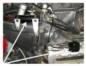
The **Control Switch (5)** is mounted on the left hand (clutch) master cylinder fluid reservoir cap. New screws are supplied to replace two of the existing reservoir cap screws. The switch is located just above the left switch block as shown in the photo at right. This bracket is stainless steel, but is now finished in black satin powder coat to better match the finish on the bike's clutch fluid housing.
