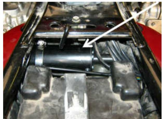
The **CIU (3)** is under the air box, in between the banks of carburetors. It attaches to the front of the pair of braces that run between the two rows of the carburetors and has a new **cable (4)** running from it to the carburetors. Some versions of the bike have an air control valve, which controls the flow of air into the exhaust system. This valve must be relocated about 1/2" to the left and rearward. A new hose is provided in the kit to enable this.
