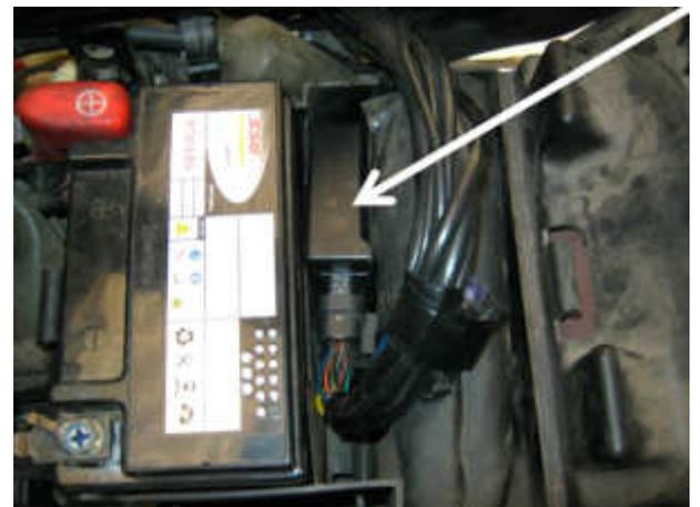
The **Electric Throttle Servo (2)** is under the rear of the fuel tank, immediately in front of the battery. The mounting bracket uses one of the existing battery box mounting bolts.
