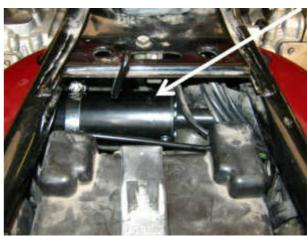
The CIU (3) is under the air box, in between the banks of carburettors. It attaches to the front of the pair of braces that run between the two rows of the carburettors and has a new **cable** (4) running from it to the carburettors. Some versions of the bike have an air control valve, which controls the flow of air into the exhaust system. This valve must be relocated about 1/2" to the left and rearward. A new hose is provided in the kit to enable this.
