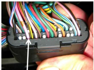
This photo shows the smaller 26-way plug from the earlier model. On this model the cruise will be connected to the light green/red wire in position 5.
