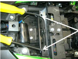
Lift the ECU up to disengage the posts from the rubber carrier.
