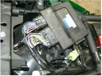
The cruise control will source speed signal (road speed) from this connection.
