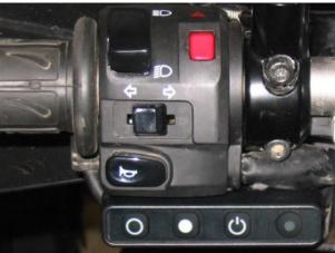
The New Slim **Control Switch (5c)** mounts on the handlebar on the left side beside the bikes' switch block, between the switch block and the clutch lever mount. This switch also has back lit buttons for night use, and an indicator light for power (ON-OFF) and engage indication.
