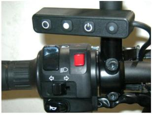
The same **Control Switch (5b)** may also be mounted below the handlebar to the left-hand (clutch) master cylinder handlebar clamp. The bracket mounts between the bottom faces of the clamp and the master cylinder. The clamp must have about  $1.5\sim2$ mm ( $0.060"\sim0.080"$ ) filed from the bottom face to allow for the thickness of the switch bracket.
