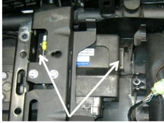
Use two suitable levers such as larger flat blade screwdrivers to lever the fender down about 10mm (3/8").
