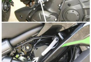
The **Electric Throttle Servo (2)** is mounted on the bike's frame tubes on the left side of the bike, next to the cylinders. It is mounted using hose clamps and rubber blocks, between the servo and the frame tubes.
