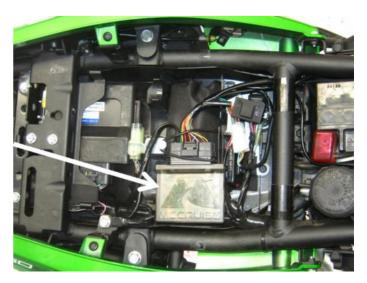
The **Actuator or throttle servo** from the old kit is now obsolete, seen here mounted on the left side of the engine bolted to the bike's frame.
