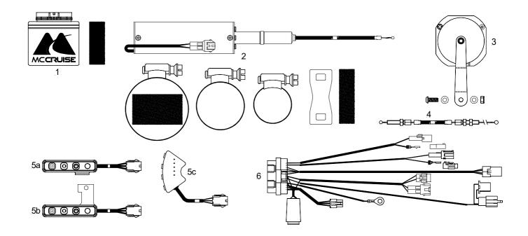
NOTE: - The installation of the cruise control requires some experimentation when mounting the new throttle servo on the bike. A variety of hose clamps and mounting brackets are provided in the kit to assist in mounting the new servo in the same or similar location that it is mounted on the new model Versys 650.
