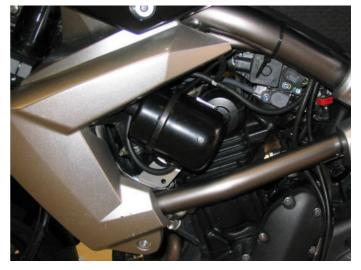
The vacuum servo has been replaced by the new **Electric Throttle Servo (2).** On the new Versys it is mounted on the bike's frame tubes on the left side of the bike, next to the cylinders. It is mounted using hose clamps and with rubber blocks between the servo and the frame tubes on the new model Versys.
