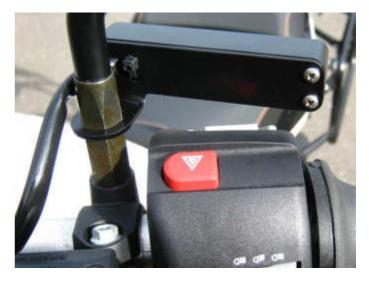
There is also an optional switch mounting bracket available (3) that places the switch roughly 10 mm (3/8") higher. This makes access to the upper arrow menu button easier, but also makes the reach to the cruise control buttons longer.
