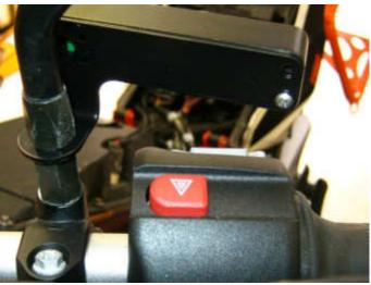
There is also another optional switch mounting bracket available (4) that places the switch below the handlebar.
