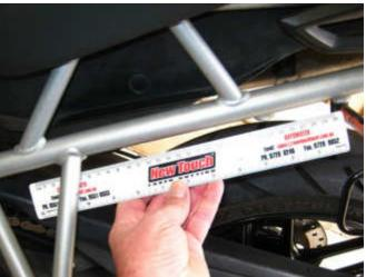
Take care with pannier frame/mounts, you will have to avoid those if the servo is to be mounted towards the back of the bike. The plastic body work around the back of the bike may also cause issues with mounting the servo further back.
