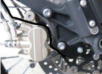
The **Speed sensor (5)** is mounted below the right hand front brake caliper. Nickel-plated magnets are placed in the heads of the bolts that mount the brake disc.
