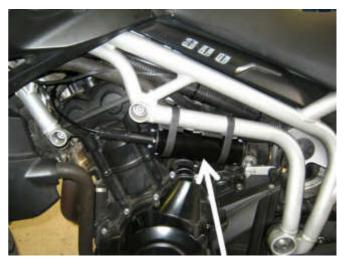
On the Tiger 800 XC, the **Electric Throttle Servo (2)** must be fitted to the lower frame tube on the rear sub-frame using hose clamps to attach it to the frame. The positions of the servo along the tube can be selected. The servo can be mounted directly above the passenger foot rests (photo left below) or further back along the tube (photo right below).
