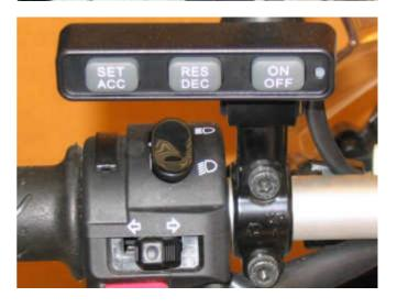
The Control Switch (6) is mounted to the left hand mirror stalk.
