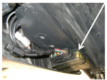
The Electric Throttle Servo (2) and the CIU or Cable Interface Unit (3) are mounted on the right side of the bike and are mostly hidden from sight.
