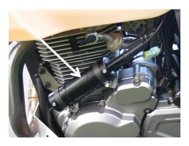
The CIU or Cable Interface Unit (3) is mounted on the right side of the motor, behind the oil cooler. It has a new cable (4) running from it to the carburetor. The mounting bracket t for the CIU has three different mounting holes for the CIU so it can be adjusted up or down to allow for different fuel tank designs. A new longer high tensile bolt is provided in the kit to replace the original bolt.
