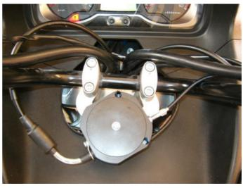
The **Control Switch (6)** is mounted to the left-hand brake master cylinder handlebar clamp. The bracket mounts between the bottom faces of the clamp and the master cylinder. The clamp must have about 1~1.5mm (0.040"~0.060") filed from the bottom face to allow for the thickness of the switch bracket. The handlebar cover must have a small section cut out to allow for the switch mounting bracket, see the photos below. More detail about this alteration is at the end of this document.
