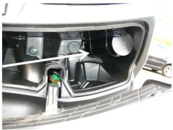
The CIU or Cable Interface Unit (3) is mounted under the handlebar cover, attached to the handlebar clamps.
