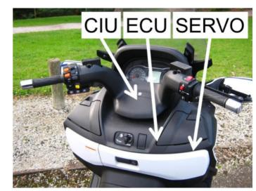
The ECU or Computer (1) is fitted on top of the main fairing storage compartment 'roof'. It is mounted using Hook & Loop (Velcro) mounting tape. The photo shows the computer on top of the main storage compartment.
