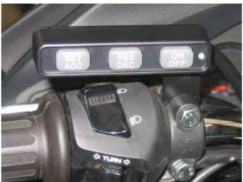
The optional **Low Control Switch mount (5b)** is shown here, below the handlebar, mounted on the clamp that mounts the clutch lever, however care must be taken with this with standard handlebars.
