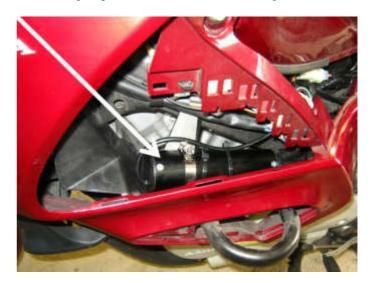
The Cable Interface Unit (3) is located above the engine. It is hidden under the air filter housing. A new cable (4) connects it to the throttle bodies.
