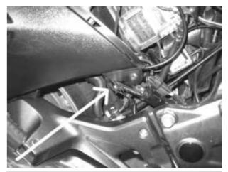
This connector is a black unsealed type connector. Both wires from the switch are black. If you follow the wires they will go down to the switch on the rear brake mechanism.
