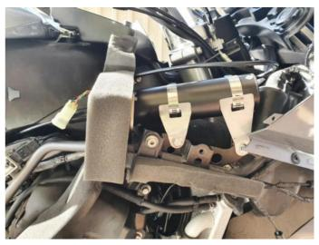
The **Cable Interface Unit (3)** is located on the left side of the motor, near the front left corner of the engine. It has a new **cable (4)** running from it to the fuel injection throttles. The computer (1) is also shown in the photo below left. The photo below right shows the CIU with the fairing fitted to the bike.
