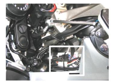
The **Throttle Servo (2)** mounts under the right-side fairing inner panel, beside the right fork leg.
