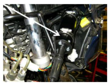
The CIU (3) is located near the front corner of the cylinder head, under the front of the air filter housing. A new **cable (4)** connects it to the throttle bodies.
