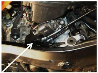
The **Control Switch (5)** is mounted below the handlebar. The bracket is mounted to the left hand (clutch) master cylinder handlebar clamp. The bracket mounts between the lower faces of the clamp. The clamp must have about  $1\sim1.5$ mm (0.040"  $\sim 0.060$ ") filed from the lower face of the clamp to allow for the thickness of the switch bracket.
