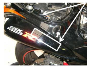
If the bike is fitted with a charcoal canister (or some other device) in this location, the servo can be mounted on the left side instead. NOTE: - This MUST be specified when the cruise control is ordered, as the cable from the servo is a different length depending which version is fitted.
