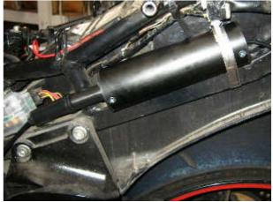
The Cable Interface Unit (3) is located below the right end of the throttle bodies, below the throttle position sensor. It has a new cable (4) that connects it to the fuel injection throttle bodies.
