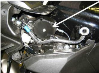
The **Speed sensor** (5) is mounted on the right of the rear wheel, behind the ABS wheel speed sensor. Nickel-plated magnets are placed in the heads of the bolts that mount the brake disc.
