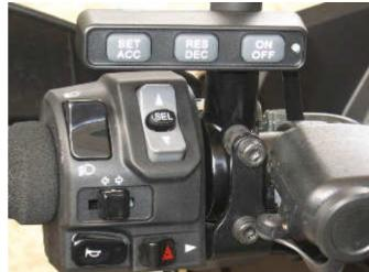
If you wish to mount the **Control Switch (6b)** below the handlebar, a replacement control switch bracket can be supplied in the kit at no extra cost.
