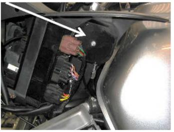
On bikes without ABS brakes, the Cable Interface Unit (3B) is mounted on the fairing frame on the right side, below the fairing storage pocket. The mounting bracket is clamped to the frame using hose clamps. It has a new cable (4) running from it to the throttle bodies.
