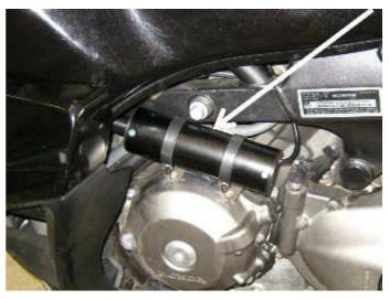
On bikes with ABS brakes, the **Cable Interface Unit (3A)** is mounted on the left side of the bike, on the bike's ECU mounting bracket, inside the fairing, in front of the fuel tank. It has a new **cable (4)** running from it to the throttle bodies.
