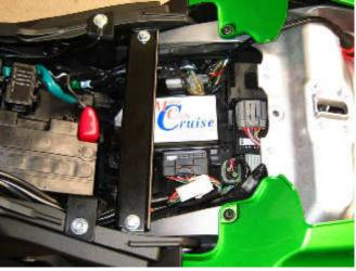
The Electric Throttle Servo (2) mounts under the right side fairing panel. A cable runs from the servo to the Cable Interface Unit.
