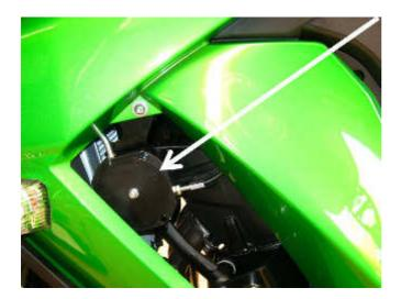
The **Speed sensor (5)** is mounted on the right of the rear wheel, in front of the ABS wheel speed sensor. Nickel-plated magnets are placed in the heads of the bolts that mount the brake disc.
