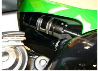
The **Cable Interface Unit (3)** is located on the left side of the motor, near the front left corner of the engine, behind the radiator. It has a new **cable (4)** running from it to the fuel injection throttles. The photos show the CIU with the fairing panels fitted and removed.
