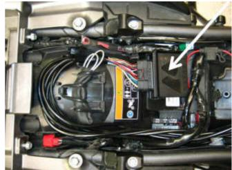
The **Electric Throttle Servo (2)** (left arrow in the photo) is mounted on the right side of the bike, on the frame tube next to the passenger footrest.
