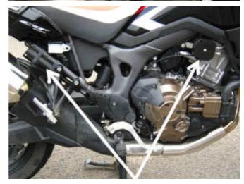
The Electric Throttle Servo (2) is mounted on the right side of the bike, on the frame tube next to the passenger footrest. A cable runs from it to the CIU (next photo).
