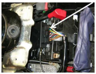
The **Electric Throttle Servo (2)** is usually mounted on the right side of the bike, on the frame, under the side cover panel below the passenger seat. A cable runs from it to the CIU (next photos).
