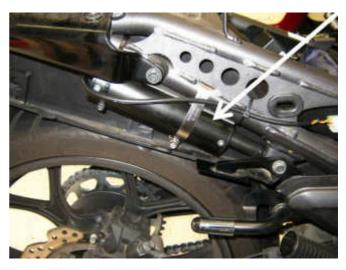
Alternatively, the throttle servo may also be mounted on the left side of the bike, next to the motor if desired. The servo is visible in this location, but is not prominent. Installing it here is slightly easier, as you don't have to remove the plastic panel below the seat on the right side, however removing this panel is a couple of minutes work.
