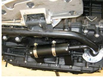
The CIU (3) is located on the left side of the bike, between the radiator and the throttle bodies, below the coolant header tank.
