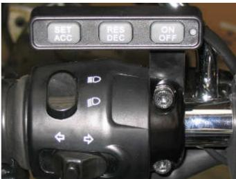
The two photos below are of the later design Triumph Touring switch gear. In this case the standard arrangement is to mount the switch above the bars (High mounting), using the same cruise control switch bracket as is used on the earlier models.
