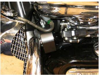
The **Control Switch** (5) is mounted to the left hand (clutch) master cylinder handlebar clamp and may be mounted below the left hand switch block (Low mounting). There are two different designs of switch gear on Rockets. This photo shows the earlier design on the Classic. See over the page for the later version of Rocket switch gear on the Touring.
