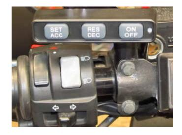
The optional Control Switch (5B) is mounted on the left hand (clutch) lever mount, and is mounted below the left switch block.
