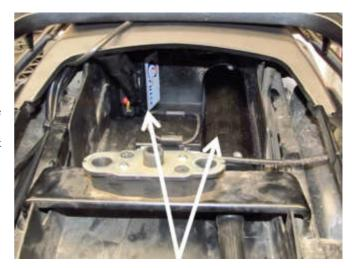
The CIU or Cable Interface Unit (3) is mounted on the left side of the bike, beside the 'V' in the cylinders. It has a new cable (4) running from it to the throttle bodies.
