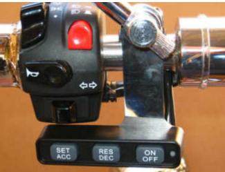
Later models have the mirror screwed directly into the handlebar. **The Control Switch (7)** in this mounting arrangement uses the 'Above Handlebar – Mirror Stalk' bracket.
