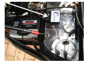
Self-adhesive 'hook & loop' (Velcro) fastener is provided in the cruise control kit to mount the **computer** on top of the fuel tank.
