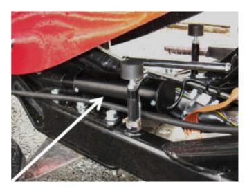
On earlier models of the Boom Auto, the servo cable went directly to the vehicle twist grip position sensor. The cable on the left (white arrow) is the original cable from the twist grip to the throttle sensor, the cable on the right is the new cable from the throttle servo. To our knowledge, this was subject to a recall and a new throttle sensor 'box' was fitted to replace this arrangement. This cruise control kit will NOT fit on this type of throttle sensor setup.
