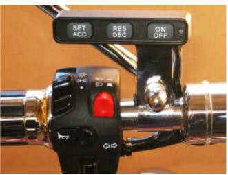
Alternatively, the **Control Switch (6b)** may be mounted below the handlebar on bikes with a clamp mounted mirror. This mounting arrangement uses the 'Below Handlebar – Mirror Clamp' bracket.
