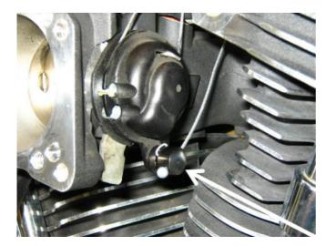
A cable runs from the throttle servo to the bike's EFI throttle body. The throttle body has a small shouldered nipple on it. This is on the side of the throttle body, where the bike's throttle cables attach to the throttle spindle. It moves with the throttle spindle when the twist grip is operated.
