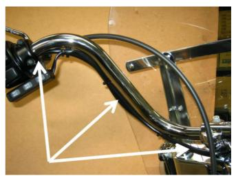
Route the cord from the handlebar (left arrow) down through the hole in the top triple clamp or triple tree (right arrow).
