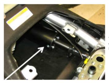
The Electric Throttle Servo (2) is mounted in the rear storage compartment. Hook & Loop (Velcro) mounting tape is used to mount the servo.
