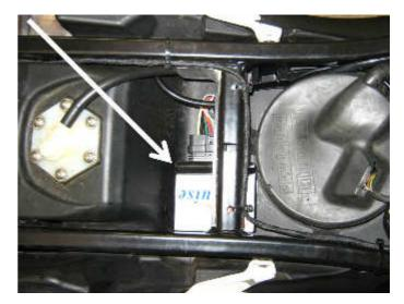
The **Electric Throttle Servo (2)** is mounted to the frame on the right side.
