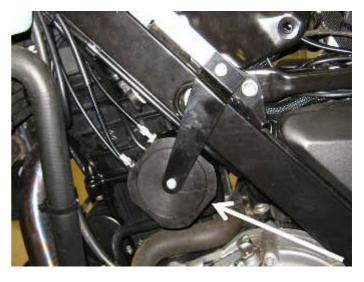
The **Speed sensor** (5) is mounted below the left side of the rear swing arm. The speed sensor detects wheel speed from the slots in the ABS tone wheel (photo below left).
