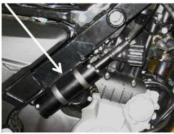
The **CIU** or **Cable Interface Unit** (3) is mounted on the left side of the bike. It has a new **cable** (4) running from it to the throttle bodies
