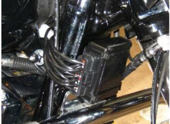
The **Electric Throttle Servo (4)** is our new 'compact' motorcycle throttle servo. It is mounted to the left side frame down tube, in front of the motor.
