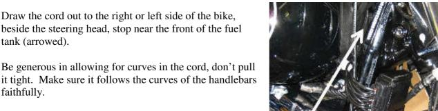
If you intend to put the switch wire INSIDE the handlebar tube (many customers do this) allow enough additional length of wire for it to enter the handlebar. This will probably use an extra 5 to 10cm (2" to 4") of wire length, depending on where the holes for the wires are in the handlebar.
