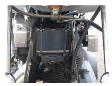
The **Computer Mounting Bracket (3)** shown here is for bikes with engine protection 'crash' bars.
