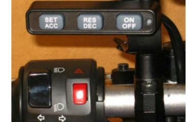
The Control Switch (5) is mounted on the left side mirror stalk.
