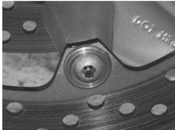
Some current (2008) bikes have flat head bolts. The recess in the head of this bolt is a T-30 'Torx' fitting and the magnets we have to fit this are 4mm diameter x 5mm long. We have seen this bolt in new (2008) R1200GS.
