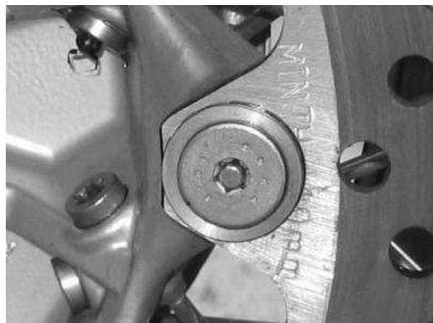
We have recently seen this new bolt, also a T-30 'Torx' fitting and uses the 4mm diameter x 5mm long magnet. We have seen this on a new (2009) F800GS. This design has gone back to the earlier practice of having a disc carrier bolted to the wheel and then the disc 'floats' on the carrier.
