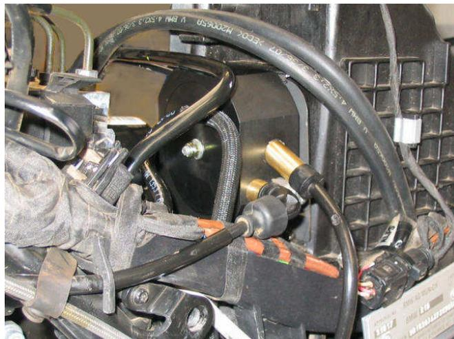
The **Speed sensor (4)** is mounted below the right hand front brake caliper. The original caliper mounting bolt is removed and a new bolt and spacer washers fitted to allow the speed sensor to be mounted. Nickel-plated magnets are placed in the heads of the bolts that mount the brake disc. **NOTE: - See the note at the end of this document regarding different magnet sizes in BMW brake disc mounting bolts.**
