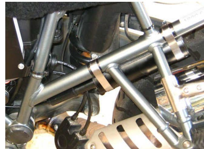
The **Electric Throttle Servo (2)** is clamped to the frame on the left side, next to the bike's rear suspension spring/damper (shock absorber).
