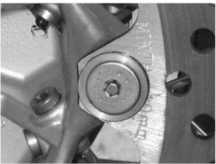
We have recently seen this new bolt, also a T-30 'Torx' fitting and uses the 4mm diameter x 5mm long magnet. We have seen this on a new (2009) F800GS. This design has gone back to the earlier practice of having a disc carrier bolted to the wheel and then the disc 'floats' on the carrier.
