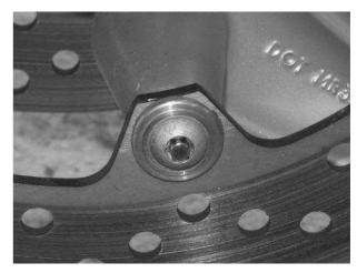
Some current (2008) bikes have flat head bolts. The recess in the head of this bolt is a T-30 'Torx' fitting and the magnets we have to fit this are 4mm diameter x 5mm long. We have seen this bolt in new (2008) R1200GS.
