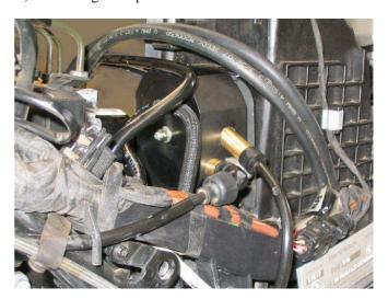
The **Speed sensor (4)** is mounted below the right hand front brake caliper. The original caliper mounting bolt is removed and a new bolt and spacer washers fitted to allows the speed sensor to the mounted. Nickel-plated magnets are placed in the heads of the bolts that mount the brake disc. **NOTE: - See the note at the end of this document regarding different magnet sizes in BMW brake disc mounting bolts.**
