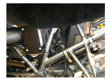
The bike's original throttle cable splitter box (throttle cable divider) is removed from the bike and our **Cable Interface Unit (3)** is fitted to the bike. No modifications to the bike's cables are required at all, it is a straight swap.
