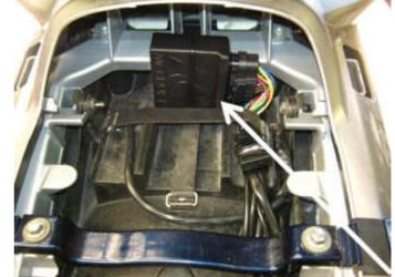
The Electric Throttle Servo (2) is bolted inside the storage compartment under the rider's seat. It does not impact on the seat height adjustment mechanism. Note that it will be necessary to cut a notch out of the air filter cover panel to clear the servo nose and cable (see photo below right).
