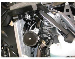
Note: - The routing of the cables around the clutch fluid line is slightly different compared to the standard routing.
