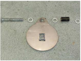
Fit the CIU bracket to the bike with the new longer bolt, washers and spacer.
