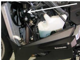
Remove the upper mounting bolt on the engine bar, as you would normally if the bar was not fitted.
