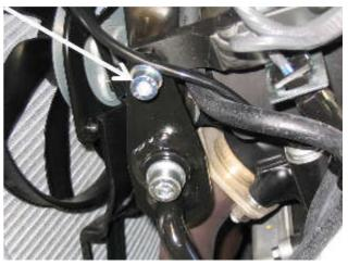
Use the new bolt, washers and spacer provided to mount the CIU mounting bracket. Fit them to the bike in the order shown in the photo.
