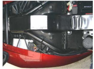
The Actuator (2) is bolted to the front of the motor beside the oil filter, using one of the starter motor mounting bolts and a lug on the oil pan. NOTE: - Some overseas models have a carbon evaporative emissions canister mounted in this location. This will have to be moved in order to fit the cruise control. A vacuum hose assembly (3) is provided to connect the actuator to the engine.
