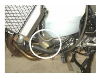
• The early (2002 without ABS) bike used to prototype the cruise control used square section unsealed connectors as shown in this photo. We will call these connectors Type 1.
