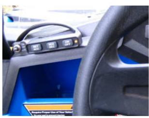
The Control Switch (2) can also be mounted on top of the dashboard on the right of the steering wheel. The photo below left shows the control switch on the Ranger XP without the optional spray power control switch. The photo below right shows the control switch fitted to another Polaris model WITH the optional spray power control switch.
