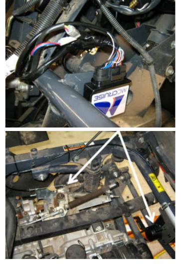
The Electric Throttle Servo (2) is mounted inside the engine bay on the rear, shown by the right arrow in the photo. A Servo Cable (3) connects the throttle servo to the vehicle's throttle mechanism (see next page) shown by the left arrow. A closer photo of the Electric Throttle Servo.
