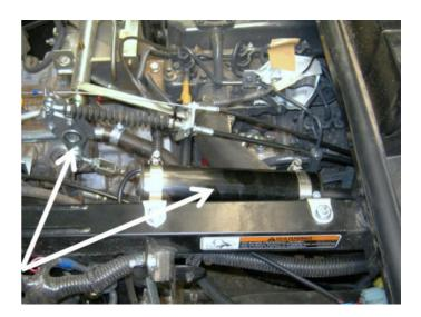
The **Throttle Lever (4)** is located on the right side of the transmission and controls the vehicle's hydrostatic transmission and engine. The new lever and other hardware bolt directly to the vehicles throttle mechanism.
