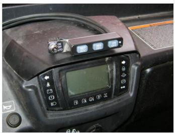
The Wiring Harness (6) is dedicated to the vehicle. Power for the cruise control is sourced from one of the vehicle's accessory power connectors. Brake sensing is sourced from the brake light switch. Neutral gear position sensing is sourced from the vehicle's neutral switch. Speed signal is sourced from the vehicle's speedometer sender. Earth (ground) is sourced from the battery negative terminal.
