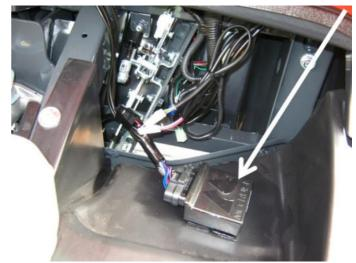
The Electric Throttle Servo (2) is mounted inside the engine bay on the right side, shown by the lower arrow in the photo. A Servo Cable (3) connects the throttle servo to the vehicle's throttle mechanism (see next page) shown by the upper arrow.
