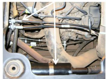
A clearer photo of the Electric Throttle Servo.
