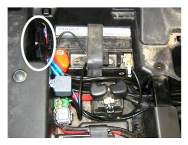
The Electric Throttle Servo (2) is fitted on the right side of the vehicle, in front of the right rear wheel, beside the air filter housing. It is clamped to the frame. A Servo cable (3) connects the throttle servo to the CIU (see below).
