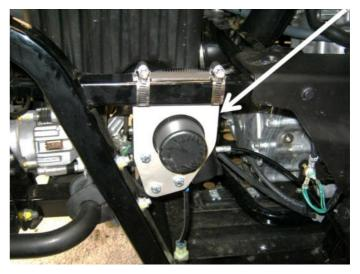
The **Cable Interface Unit (4)** is located behind the passenger seat, beside the engine and has a new **cable (5)** running from the CIU to the throttle body. The existing throttle cable is disconnected from the throttle body and is connected to the CIU. The CIU 'translates' throttle trigger movement and throttle servo operation to the vehicles throttle body.
