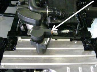
The **Cable Interface Unit (4)** is located behind the passenger seat and has a new **cable (5)** running from the CIU to the throttle body. The existing throttle cable is disconnected from the throttle body and is connected to the CIU. The CIU 'translates' throttle trigger movement and throttle servo operation to the vehicles throttle body. The photo below left shows the CIU with the rear body panel and rack in place. The photo below right shows the CIU with the panel and rack removed.
