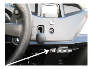
The **Wiring Harness** (7) is dedicated to the vehicle. Power for the cruise control is sourced from the vehicles brake light switch connector. The brake light switch is disconnected and matching plugs on the speed limiter loom are connected to the vehicle's plugs. Neutral gear position detection is sourced from the vehicles neutral switch circuit. Speed signal is sourced from the vehicle's speedometer sender. Ground is sourced from the negative terminal of the battery.
