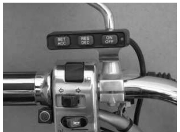
BMW R1200GS – note that access to trip and hazard light switches is restricted but is still possible from behind the cruise control switch.
