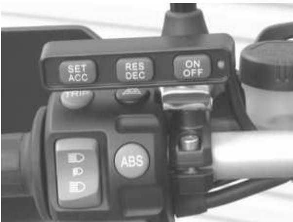
BMW R1200GS – note that access to trip and hazard light switches is restricted but is still possible from behind the cruise control switch.
