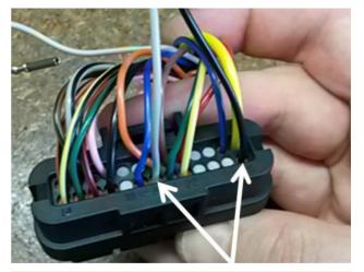
Check that the inserted terminals are pushed in all the way.
