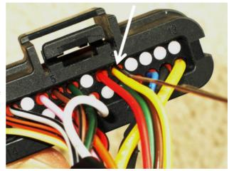
Push the two white tabs down to close the terminal lock.
