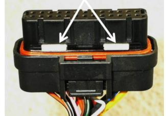
Gently pull the grey brake sensor wire (terminal hole 20) out of the plug (left arrows).
