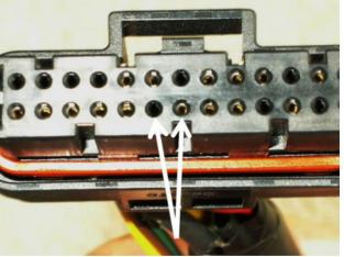
If any terminals are not fully home, use the paper clip to push the terminal in all the way.
