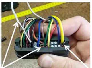
Insert the terminal on the grey wire from the supplied 'patch' into terminal hole 20 (left arrow).
