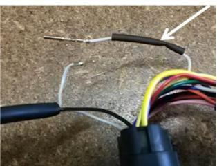
Connect the terminals on the grey wires from the patch and the cruise harness.
