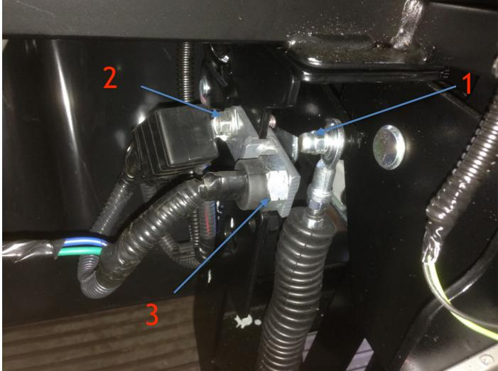
3. Next, disconnect the key switch multi-wire connector from the switch by squeezing the locking tab and gently pulling the plug away from the switch (4)
