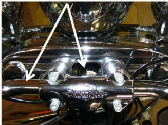
Draw the cord out to the right or left side of the bike, beside the steering head, stop near the front of the fuel tank (arrowed).
