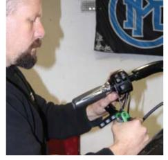
2 Craig now installs the control switch block below the left handlebar switch block and then routes the switch wiring through the handlebars.
