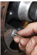
4 And then places each of the supplied magnets into the heads of the front disc brake mounting bolts.
