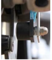
5 Here we see the speed sensor set up with the specified gap of between one and three millimetres between the sensor face and
