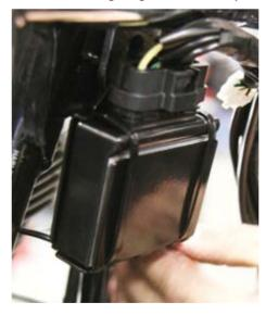
7 He now fits it to the front of the frame. Normally it would be mounted up the other way with the wires emerging from the bottom, rather than the top. However, on Jane's bike an aftermarket crash bar required us to (temporarily) mount it upside down. Not that this is a problem, as the electronics are enclosed in a plastic box that is filled with a rubberised compound to completely enclose the parts in a waterproof environment. The connectors are also of a totally waterproof design.
