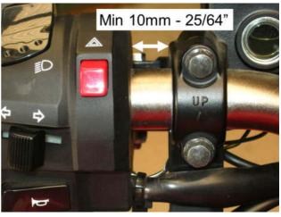
In this example the switch is mounted on the other side of the clutch lever mount, which makes for a longer reach to the buttons, but is still satisfactory.
