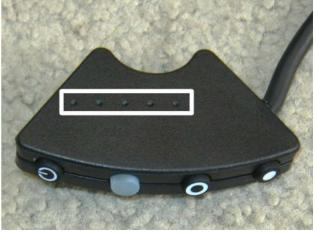
The back of the switch (outlined) may also be cut off if desired. The line shows the upper edge of the cavity for the cable tie. This material can be cut off the switch without affecting the integrity of the switch.
