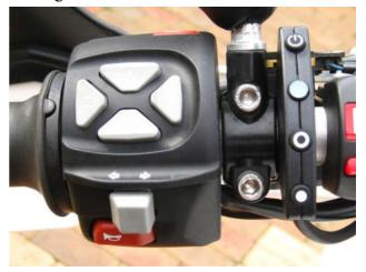
The housing has slot that runs through the switch for a cable tie, the cable tie straps the switch to the handlebar.
