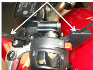
We suggest aligning the SET button roughly with the bike's indicator switch and press the switch against the handlebar, so the double sided tape holds the switch in position.
