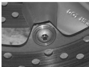
Current bikes from 2008 have flat head bolts. The recess in the head of this bolt is a T-30 'Torx' fitting and the magnets we have to fit this are 4mm diameter x 5mm long.
