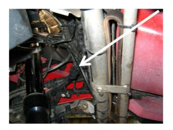
If your bike has this socket with blue/green wire (arrowed), the cruise control may be able to be connected to this wire for speed signal.
