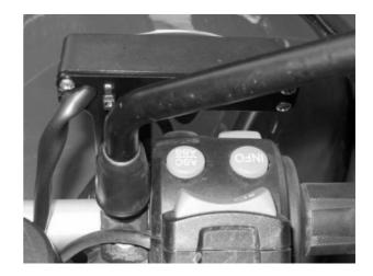
We need to know if the standard (MCS830L) medium (MCS830W) or tallest (MCS830U) switch bracket is required. We recommend the standard 9MCS830L) bracket for the best combination of access to the bike's buttons and light switch and reach to the cruise control switch.
